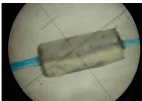
Fig. 19 Used bead of \phi 0.4mm in diameter and 1mm in length supported with a fishing thread of 50 \mu m in diameter.
